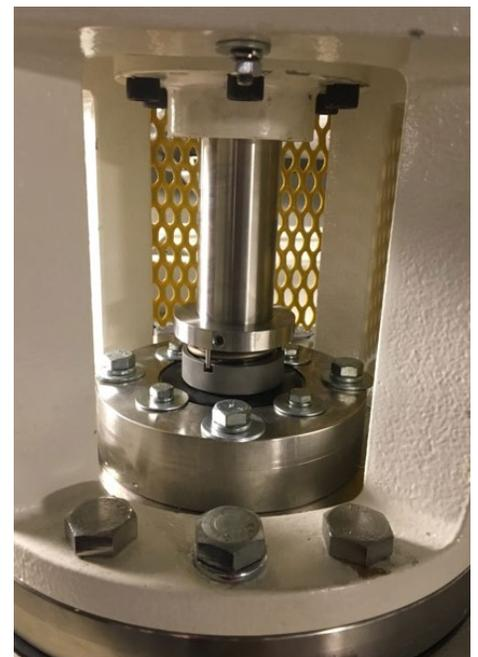
12MR seal aligned and set to proper spring load.
