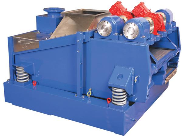
VSM 300 with fume extraction hood and flange connection for distribution (spider) feed box
